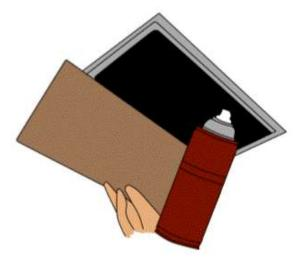
Though not necessary, we recommend using a black spray paint in your duct, otherwise you may be able to see the metal duct work.
