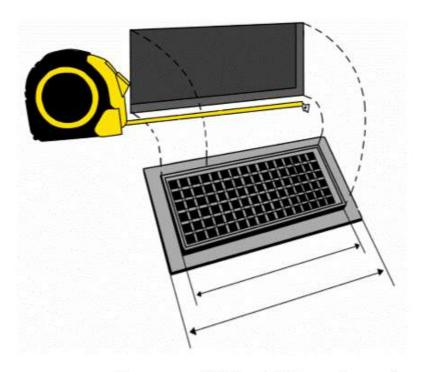
Measure your opening. Use width by height to determine the size of the grille you need, the overall size will be larger when you include the frame.
