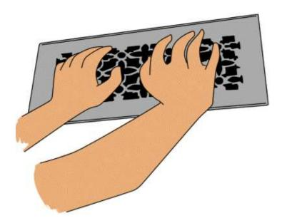
Before installing, make sure the lip of the grille (if your grille has one) fits inside of your opening and the framing fits flat with the wall or ceiling.
