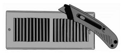
Clean around your existing grille to make it easier to remove after unscrewing. Old paint and caulking is quickly removed by running a box cutter around the grille.
