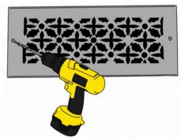
Screw your grille in using the provided screws. If you do not have pre-drilled screw holes, you may screw right through the grille or use a 23 gauge nail gun (this will provide a semi permanent application). If desired, use caulking around the grille to fill any gaps between the wall/ceiling.
